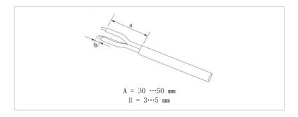
2. Disassemble the connector in accordance with the following illustration. Guide the AC output cable through the cable gland.
