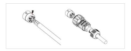
2. Connect and lock the connector by turning it clockwise.
