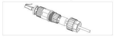
3. Lock the connector by turning clockwise:
