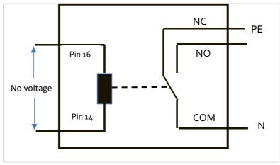
Relay mode 2 (Relay Close In EPS) switches the contact in the opposite direction, i.e. in the on-grid mode there is no voltage, in the EPS mode there is voltage.
